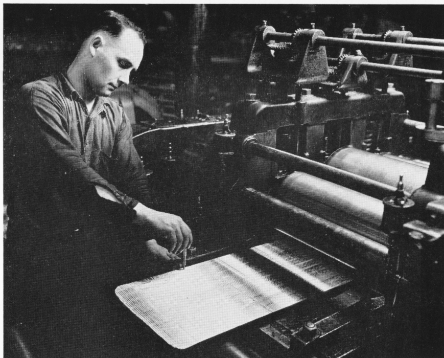
Here we see Albert Proulx of the Rolling Mill making a final test of a rolled sheet to ascertain if it has just the exact thickness required by the specifications which Scovill products live up to scrupulously.
