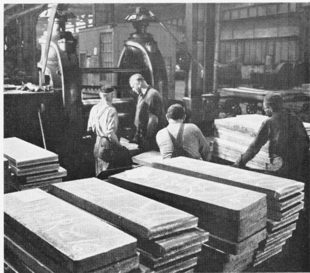
These bars as they come from the molds are of various thicknesses. The rolling mills then reduce them to the desired thickness for fabricating. Laboratory tests have meanwhile been made of the metal to make sure that it fulfills all the requirements of a perfect alloy. Scovill wants to turn out only perfect work. No defects are allowed to get by.
