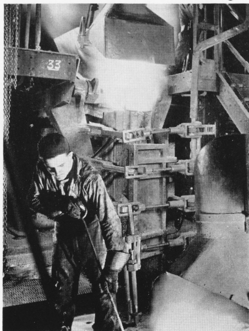
The charge of metal is placed in a melting furnace operating at a temperature of about 1,000 degrees C. and after about an hour the molten alloy is poured into molds.
