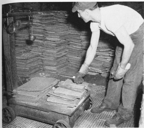
Honorius Chabot of the Casting Shop weighs up virgin copper just in from the refineries in order to make a charge for the melting furnace. Zinc and scrap will be added to the copper to make the resulting cartridge brass. This contains about 70% copper and 30% zinc. The great majority of Scovill finished products are now made of this alloy.
